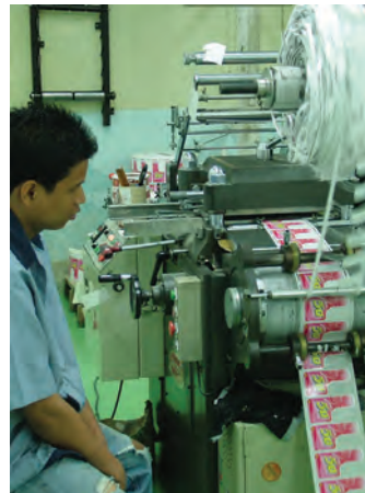
An offline die-cutter is available to process labels from the screen printing or the flat-bed letterpress machines.
