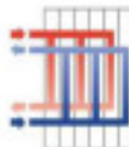
單面流適用於各種的熱傳應用 Single-pass arrangement Suitable for most application.
